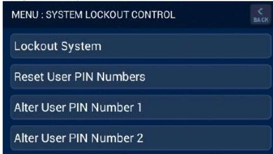
To lock the system press “Lockout System” and enter the User PIN, the default PIN is “1111” until modified. When locked a padlock icon will flash at the bottom of the touch screen.
