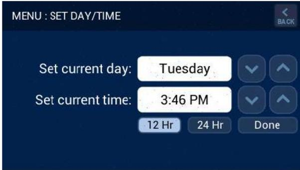
To set the Day and Time press the adjacent UP/DOWN arrows. Pressing the “Done” button saves the changes and returns you to the configuration menu screen. Pressing the “BACK” button does not save the changes and returns to the configuration menu screen.
