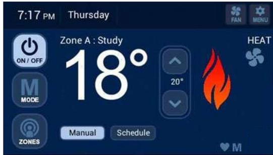
**Note:** A flashing “ZONE” button on the Home Screen indicates all Zones are satisfied and system is in standby.
