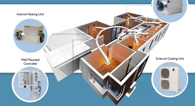
When installing a Brivis ICE<sup>TM</sup> Add-on refrigerated cooling system to an existing Ducted Gas Heating system, care must be taken to ensure the duct system is sized and designed correctly. If you are installing a heating system and plan to install Brivis ICE<sup>TM</sup> Add-on refrigerated cooling system at a later date, then ensure that you advise your dealer and they will size the system accordingly.
